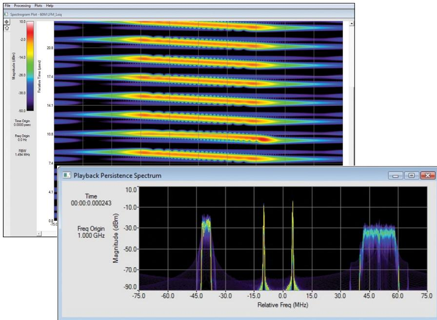
The IQC-2110 coupled with the X-COM continuous playback generator (CPG-2110) can also re-play all or any part of the recorded spectrum with full 16 bit I and Q precision using an Agilent vector signal generator. These capabilities make it possible to find critical signals of interest from within the captured data rapidly.
